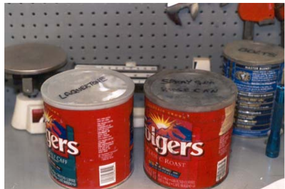
Figure 12. Containers used at Company B for cleaning spray gun parts
