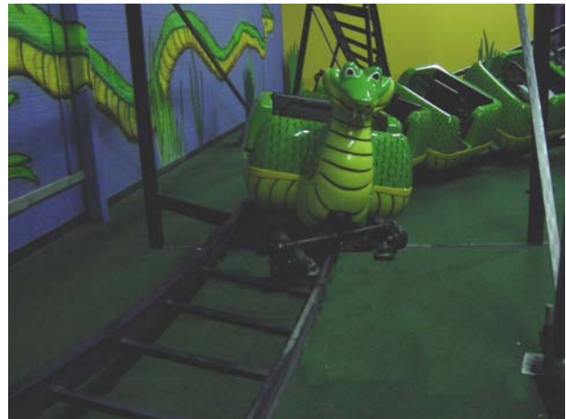
Figure 1. Derailed roller coaster
